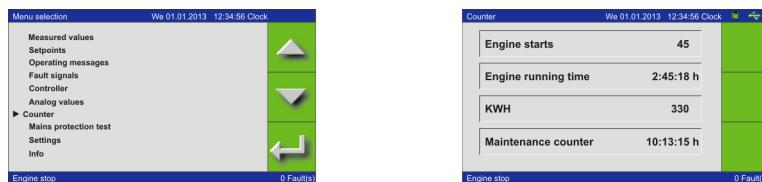
All counter values are also displayed on the start screen, with the exception of the maintenance counter. If the maintenance counter is enabled, the time will only be displayed via the counter menu.
