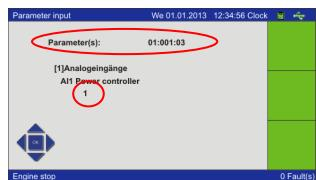
If there is no PC available all parameters can also be adjusted directly at the KOP2. The input is protected by a PIN.
