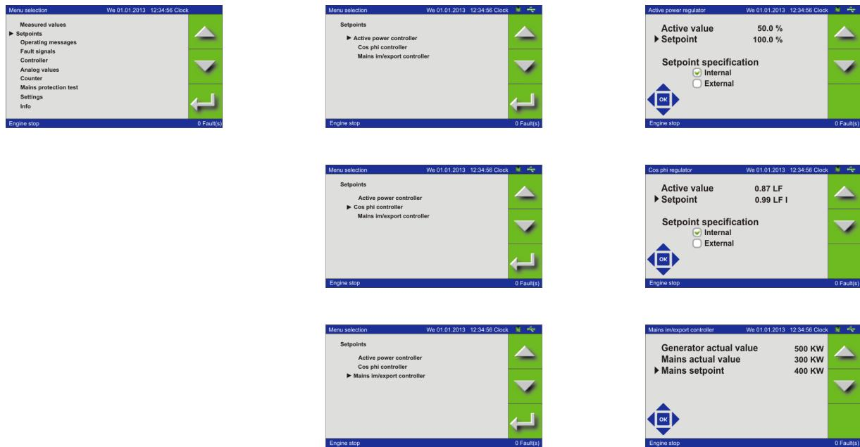
Setpoints can be set for three different regulators. For the setpoint specification selection is possible between the setpoint adjusted at the panel (internal) or the analog value (external). When not activated via parameterization the menus for these regulators are greyed out and cannot be selected.
