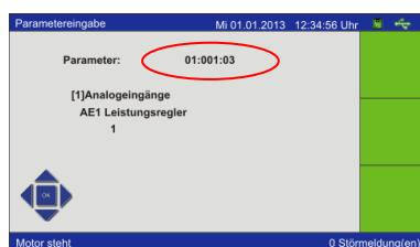
For parameter edition the menu Parameter input has to be opened in item Settings. SOP edition with the help of the cursor keys the position of the value to be modified will be selected in the upper line of the displayed dialogue.
