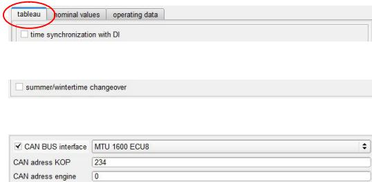
The screenshot shows a software interface with three tabs at the top: 'tableau' (highlighted with a red circle), 'nominal values', and 'operating data'. Below the tabs are two checkboxes: 'time synchronization with DI' and 'summer/wintertime changeover'. A dropdown menu shows 'CAN BUS interface MTU 1600 ECU8' and 'CAN adress KOP 234'. Another dropdown shows 'CAN adress engine 0'.
