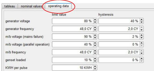
The screenshot shows a software interface with three tabs at the top: 'tableau' (highlighted with a red circle), 'nominal values', and 'operating data' (selected). The interface displays operating data with columns for 'limit value' and 'hysteresis'. For example, generator voltage has a limit value of 80 % and hysteresis of 40 %. Other parameters include generator frequency, m/b voltage (mains failure), m/b voltage (parallel operation), m/b frequency, genset loaded, and KWH per pulse.
